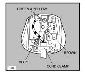
The wire coloured green and yellow must be connected to the terminal marked with the letter  $\ll E \gg$  or by the earth symbol  $\frac{1}{2}$  or coloured green and yellow.
